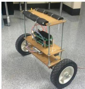
which is a senior project that allows students to study and implement digital control in real hardware. An Inertial Measurement Unit (IMU) is used as a tilt sensor and a simple PID controller is applied to regulate the target.
