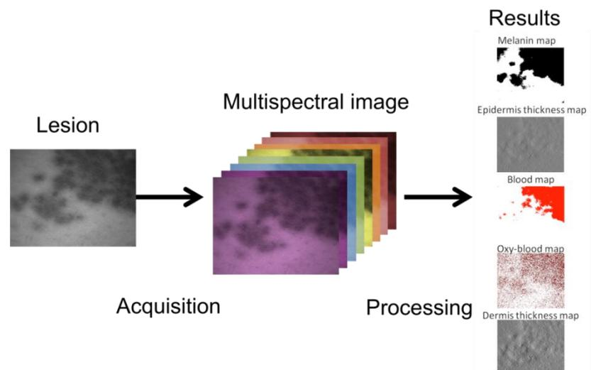
*Schematic of multispectral imaging system: acquisition + processing yielding concentration maps*
