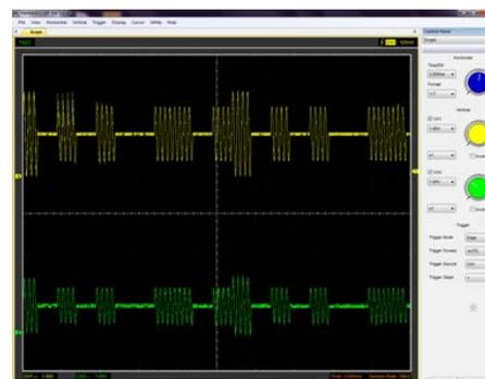
*Signals generated by our own lab kits. The top part of each figure is the transmitted signal, while the bottom is the received signal. The three modulation schemes are Pulse Amplitude Modulation (PAM), Amplitude Shift Keying (ASK), and Frequency Shift Keying (FSK).*
