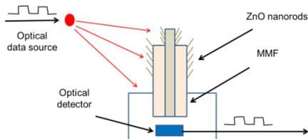
(1) Schematic view of the proposed optical antenna configuration
