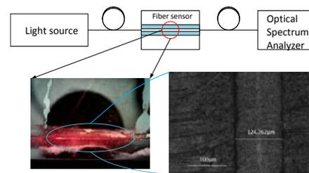
Experiment setup with microscopic image of fiber sensor surface (lower right)
