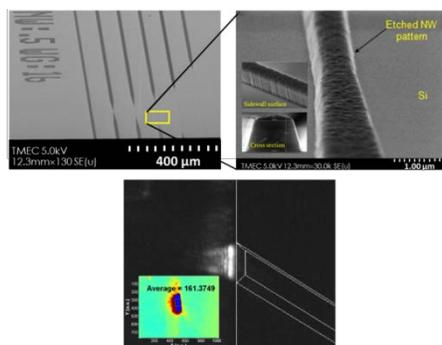
*The structure and electron microscopic images for the nano-wires used in this study.*
