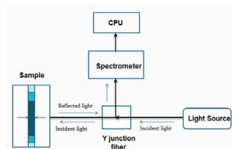
Schematic diagram of the measurement setup
