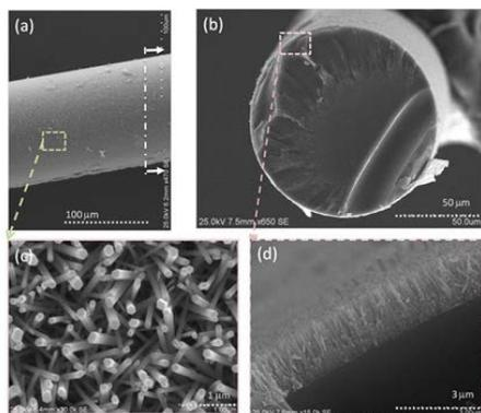
(2) SEM images of (a) Uniform growth of ZnO nanorods on the optical fibers (b) Cross sectional view of the optical fiber showing the growth thickness (c) High magnification top view and (d) Side view of the rods on the optical fiber showing the growth directionality
